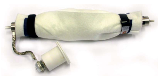
Image 8-22 Left: Xenon lamp wrapped in a protective cloth. Right: Xenon lamp captured in a protective container.
