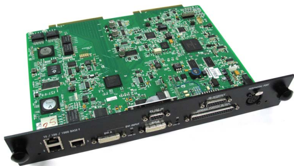
Image 15-6 Cinema controller board
