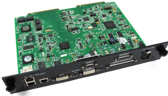
Image 13-4 Cinema controller board
