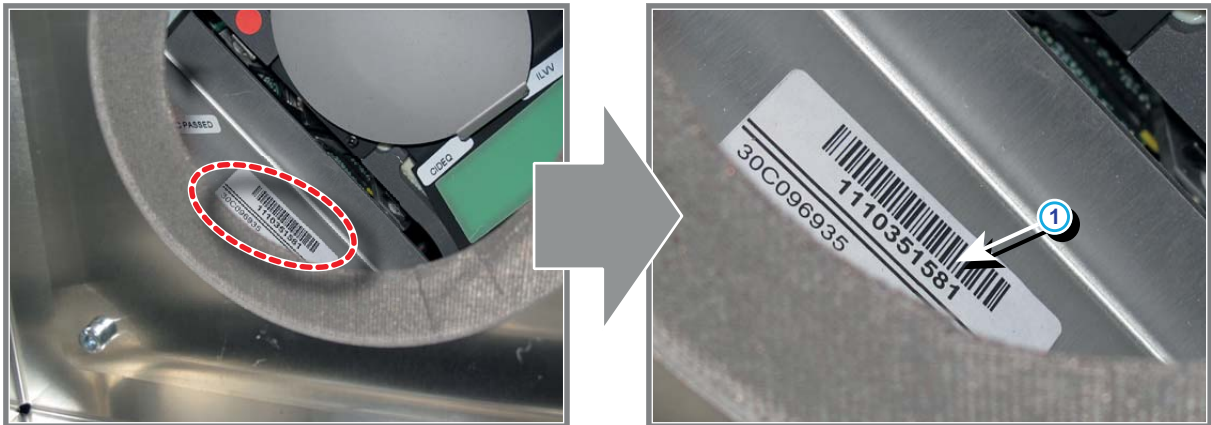
Image 9-1 Location label with Serial Number of the Light Processor of a DP4K-P projector.
