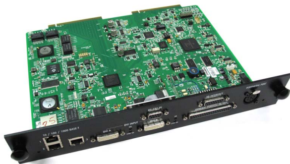
Image 15-4 Cinema controller board
