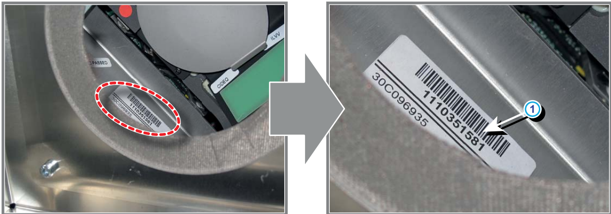
Image 14-1 Location label with Serial Number of the Light Processor of a DP4K-P projector.
